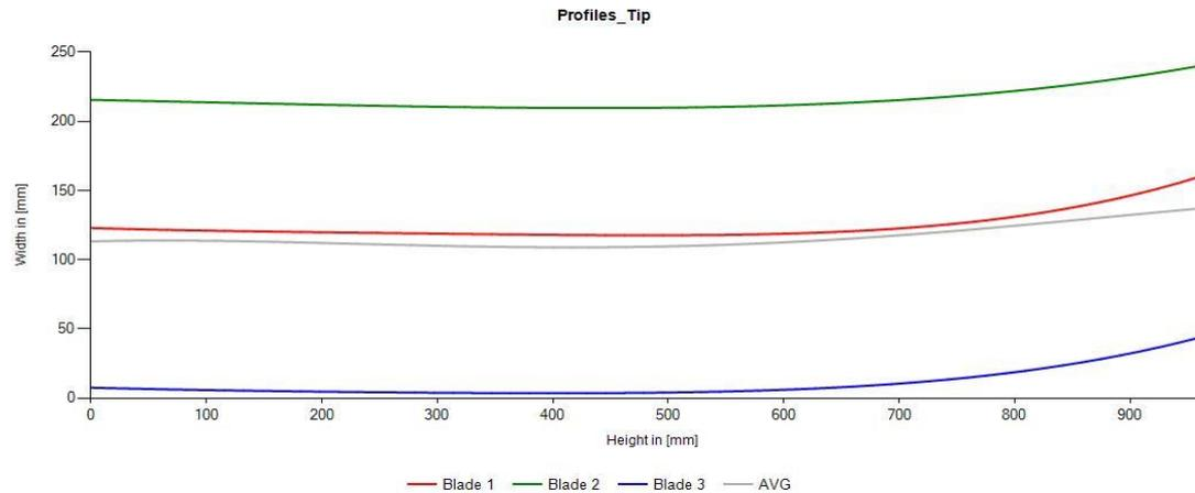
The blade tip profile graph indicate whether a blade is closer to the tower compared to the 2 other ones.
