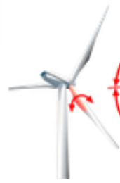
Blade angle difference of 1.2°
