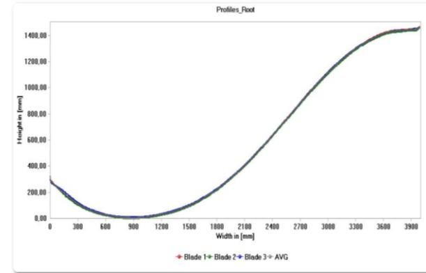
The blade angle difference is the most important result from the Romeg inspection. The 2 graphs above show the 3 blade profiles and the average one before and after correction.
