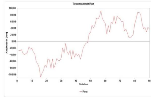
Tower vibration due to aerodynamic imbalance is usually visible starting at a 0,8° blade angle difference.
