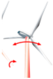
Tower vibration with 1.2° blade angle difference
